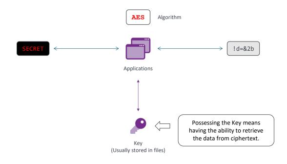
Executed by **Applications**, encryption is a method protecting sensitive data by converting it into ciphertext, using an **algorithm** and a **random** key.
